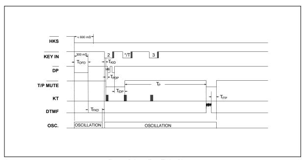
Figure 5 Pulse-to-Tone Timing Diagram
