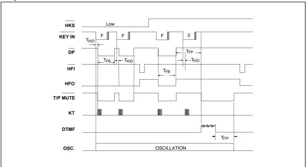
Figure 6. Flash Timing Diagram
