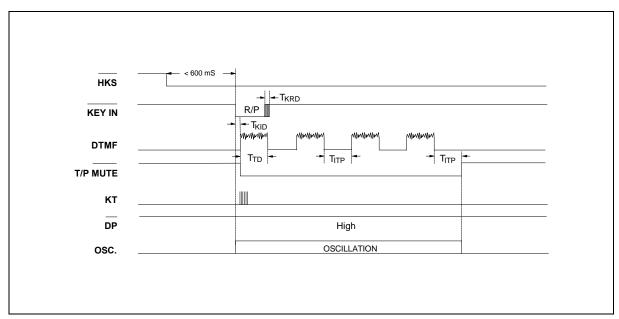
Figure 2c. Auto Dialing Timing Diagram (Tone Mode Without Lock Function)
