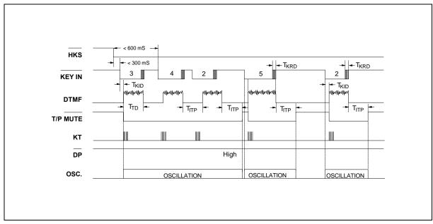
Figure 2a. Normal Dialing Timing Diagram (Tone Mode Without Lock Function)
