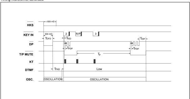
Figure 4. Pause Function Timing Diagram
