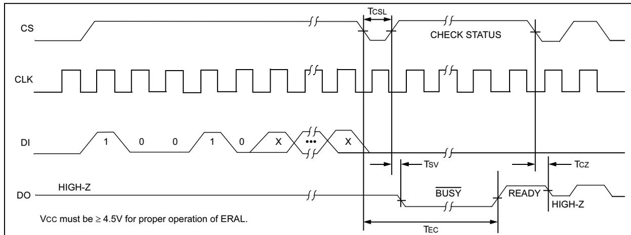
FIGURE 2-4: ERAL TIMING FOR 93C DEVICES
