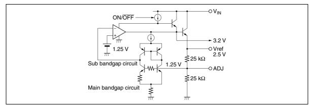
Figure 5.1 Vref Reference Circuit
