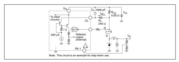
Figure 8.1 Example for Step-Down Use
