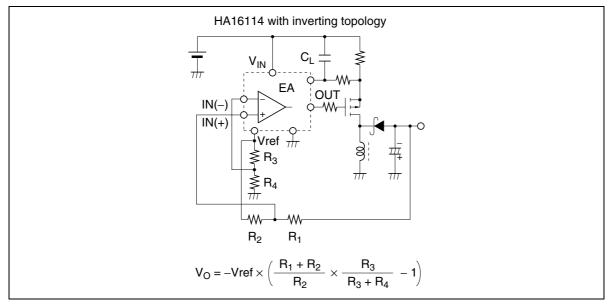
Figure 2.2 Output Voltage Setting (2)
