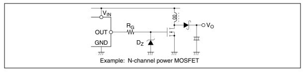
Figure 4.2 Gate Protection by Zener Diodes
