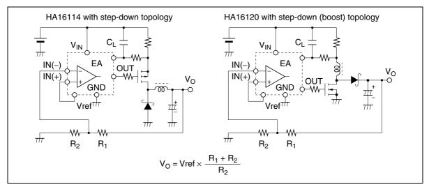
Figure 2.1 Output Voltage Setting (1)
