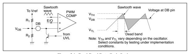
Figure 3.1 Dead-Band Duty Cycle Setting
