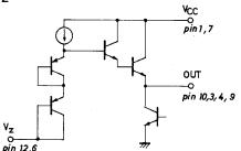
$V_{BE}$  of 2 output NPN transistors is canceled by  $V_{BE}$  of 2 PNP transistors.  $V_{o}\!\simeq\!V_{Z}$
