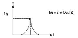
When Rd is connected to the hysteresis pin,  $(Rd + r_{cs} // Rh)$  1/g is the condition for oscillation to start, and (Rd + Rh) > 1/g is the condition for oscillation to stop. Note that  $r_{cs}$  is the internal resistance of the hysteresis pin.
