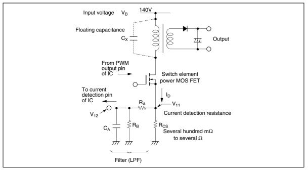
Figure 2.1 Current Detection Circuit
