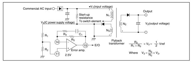
Figure 1.1 Error Amplifier Peripheral Circuitry Diagram
