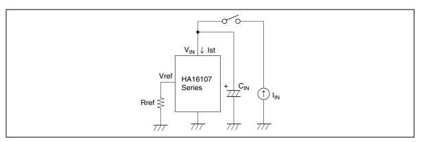
Figure 1 Standby Current Test Circuit
