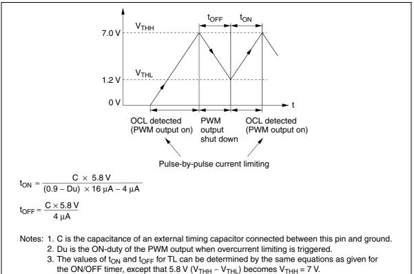
If the timer goes off during soft start or in the undervoltage lockout region, after recovery, output will come on after the soft-start time or after the rise time to the undervoltage lockout release point, which is determined by the time constant.
