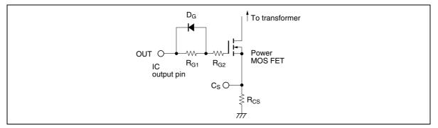
Figure 4.1 Gate Drive Circuit
