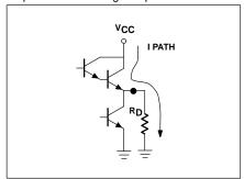
As the output frequency increases the measured current approaches that of static High outputs.
