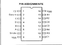
This device contains circuitry to protect the inputs against damage due to high static voltages or electric fields; however, it is advised that normal precautions be taken to avoid application of any voltage higher than maximum rated voltages to this high impedance circuit For proper operation it is recommended that Vin and Vout be constrained to the range Vss < (Vin or Vout): VDD Unused control inputs must always be tied to an appropriate logic voltage level (e.g.,
