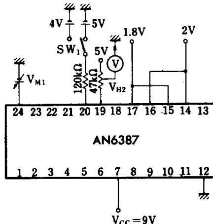
When  $S_1 = 5V$  and  $V_{M1} = 9V$ ,  $V_{M2} \cdots$  High voltage
