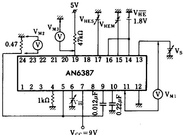
Read  $V_{M1}$  and  $V_{M2}$  when  $V_{HES} = V_{HEM} = 2V$ ,  $V_{DS} = 2V$  and  $V_s = 0 \sim 6V$ .
