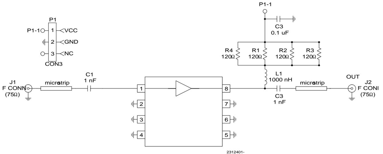
**NOTE:** For 5V applications, R1 to R4 may be removed (shorted). This will result in degraded distortion performance.
