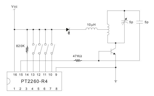
UHF Band 4-Data Transmitter Circuit is recommended.
