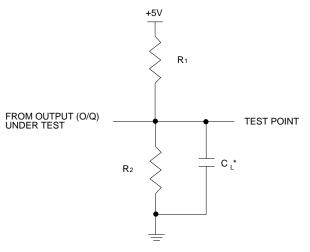
$^{\star}\text{C}_{\, \text{L}}$  INCLUDES TEST FIXTURE AND PROBE CAPACITANCE
