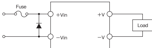
Figure1-5: Protection for Reversed Connection of Input
