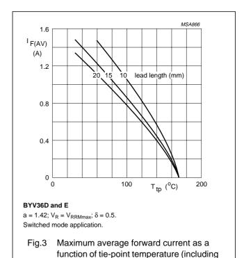
losses due to reverse leakage).
