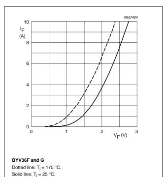
Fig.21 Forward current as a function of forward
