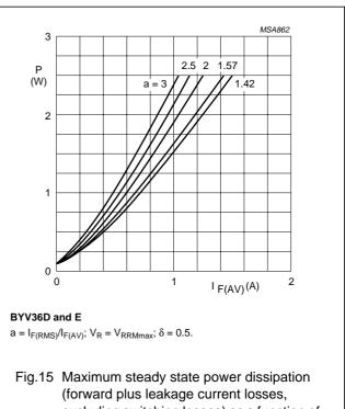
excluding switching losses) as a function of average forward current.
