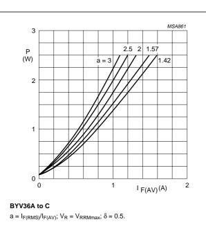
Fig.14 Maximum steady state power dissipation (forward plus leakage current losses, excluding switching losses) as a function of average forward current.
