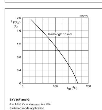
Fig.4 Maximum average forward current as a function of tie-point temperature (including losses due to reverse leakage).
