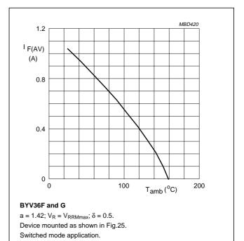
Fig.7 Maximum average forward current as a function of ambient temperature (including losses due to reverse leakage).
