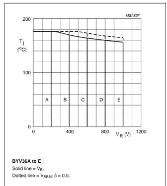
Fig.17 Maximum permissible junction temperature as a function of reverse voltage.
