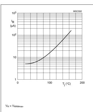
Fig.22 Reverse current as a function of junction temperature; maximum values.
