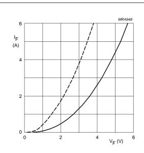
Dotted line:  $T_j = 150 \,^{\circ}\text{C}$ . Solid line:  $T_j = 25 \,^{\circ}\text{C}$ .
