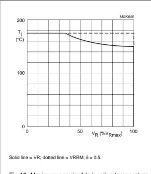
Fig.10 Maximum permissible junction temperature as a function of maximum reverse voltage percentage.
