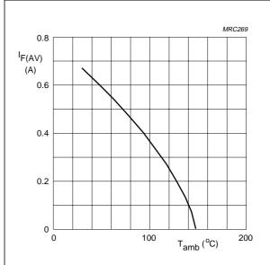
$a=1.42;\ V_R=V_{RRMmax};\ \delta=0.5.$  Device mounted as shown in Fig.11. Switched mode application.
