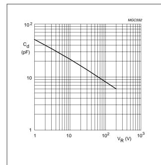
$f = 1 \text{ MHz}; T_j = 25 \,^{\circ}\text{C}.$
