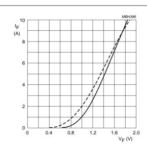
Solid line:  $T_j = 25 \,^{\circ}\text{C}$ . Dotted line:  $T_j = 175 \,^{\circ}\text{C}$ .
