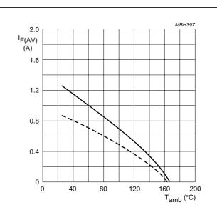
$$\begin{split} &V_R=V_{RRMmax},\,\delta=0.5;\,a=1.57.\\ &\text{Device mounted as shown in Fig.7}\\ &\text{Solid line: Al}_2O_3\text{ PCB; dotted line: epoxy PCB.} \end{split}$$
