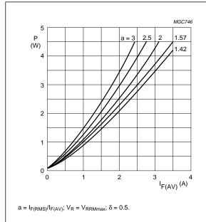
Maximum steady state power dissipation (forward plus leakage current losses, excluding switching losses) as a function of average forward current.
