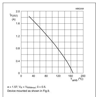
Maximum permissible average forward current as a function of ambient temperature (including losses due to reverse leakage).
