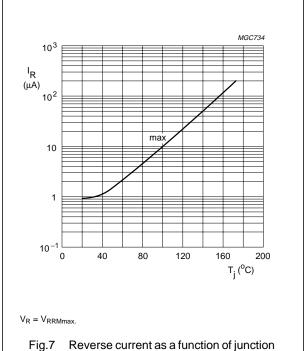
Fig.7 Reverse current as a function of junction temperature; maximum values.
