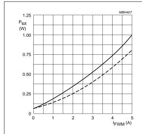
Solid line: basic high-voltage E/W modulator circuit; see Fig.8. Dotted line: basic conventional horizontal deflection circuit; see Fig.9. Curves include power dissipation due to switching losses.
