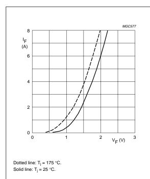
Fig.8 Forward current as a function of forward voltage; maximum values.
