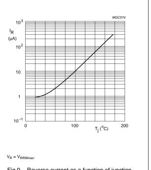
Fig.9 Reverse current as a function of junction temperature; maximum values.
