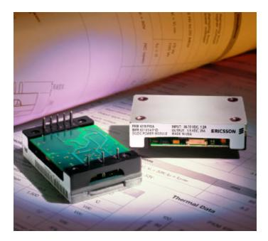
Ericsson's PKM 4000 Power Modules address the converging "New Telecoms" market by specifying the input voltage range in accordance with ETSI specifications. Included in the PKM 4000 series are over-voltage protection, under voltage protection, over temperature protection, soft-start, and short circuit protection. The PKM 4000 Series also offers the flexibility of using an optional heatsink when needed, enabling reduced airflow, extended reliability, and higher ambient temperature operation.
