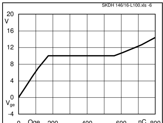
Fig. 6 Typ gate charge characteristic
