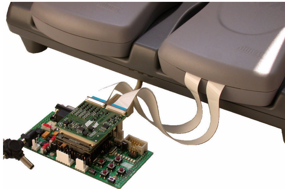
Figure 3-46 . Connecting AVR ICE 50 for Debugging
