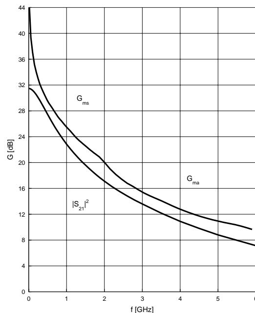
**Power gain  $G_{ma}, G_{ms} = f(V_{CE})$**
