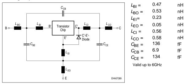
The SOT343 package has two emitter leads. To avoid high complexity to the package equivalent circuit both leads are combined in one electrical connection
