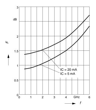
Noise figure  $F = f(I_C)$  $V_{CE} = 2 V, f = 1.8 \text{ GHz}$
