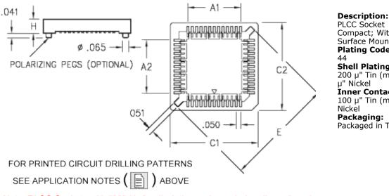
Compact; Without Polarizing Peg Surface Mount Plating Code: Shell Plating: 200 µ" Tin (matte finish) over 100 µ" Nickel Inner Contact Plating: 100  $\mu$ " Tin (matte finish) over 50  $\mu$ " Nickel Packaging:
