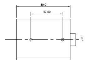
The heatsink is supplied with two mounting screws -Skt Hd M4 x12mm
