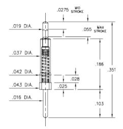
**Description:** 0950 - Spring-Loaded Pin Packaging: Packaged in Bulk
