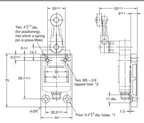
Note: Four hexagonal flat head bolts  $(M5 \times 0.8, length: 10)$ , two Allen-head bolts (M5 × 0.8, length: 15), and two spring pins  $(4 \times 14)$  are included.
