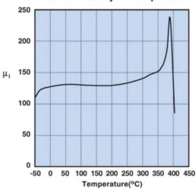
Measured on a 19/10/6mm toroid at 100kHz.
