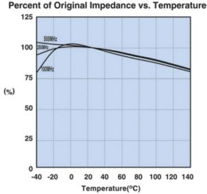
Measured on a 2661000301 using the HP4291A.
