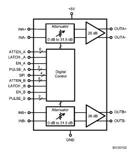
FIGURE 3. LMH6521 Block Diagram
