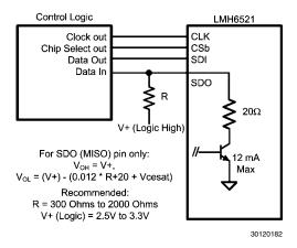
FIGURE 11. Serial Mode 4-wire Connection
