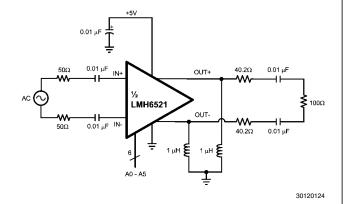
FIGURE 2. Basic Operating Connection
