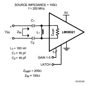
FIGURE 4. Differential 200Ω LC Conversion Circuit
