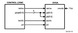
FIGURE 9. Parallel Mode Connection Using Latch Pins to Mulitplex Digital Data
