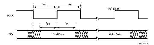
FIGURE 13. Write Timing Data Written to SDI Pin
