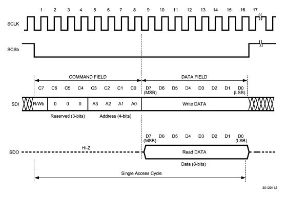
FIGURE 10. Serial Interface Protocol (SPI compatible)
