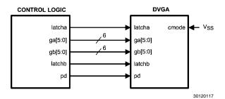
FIGURE 7. Parallel Mode Connection for Fastest Response
