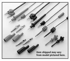
Model 5804 Test Lead Set: Designed to be used with Keithley instruments that measure 4-terminal resistance. Contains: 2 test leads, 0.9m (36 in), red and black; 2 test clips, red and black; 2 plunger clip adapters, red and black; 2 alligator clips with boots (accept standard test probe tip); 2 alligator clips with boots (barrels accept standard banana plugs).
