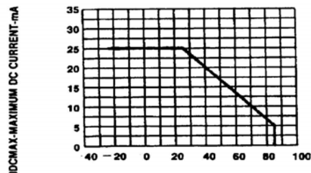
Fig.4 MAXIMUM ALLOWABLE DC CURRENT PER SEGMENT VS. A FUNCTION OF AMBIENT TEMPERATURE.
