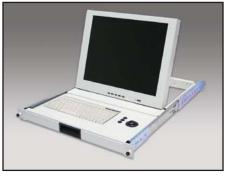
**Model 4200-FPD-RM:** High resolution, 1U (17 inch) TFT display with keyboard and trackball pointing device. Includes 4200-KEY-RM slide rack mounting kit as well as cables and accessories to connect directly to embedded KPXI controllers or the Model 4200-SCS. **Note:** Unit is not CE marked for sale in EEC countries.
