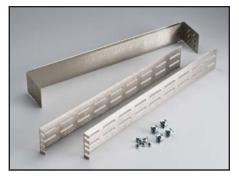
**Model 4288-10 Rear Support Mount Kit:** For rack mount applications where more than one or two card modules are installed to provide added support for the rear of the mainframe. Note that front rack mounting hardware is supplied with the Model 3706 mainframe. 88mm (3.5 in) height.
