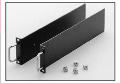
Model 1938 Fixed Rack Mount Kit: Consists of two flanged brackets and hardware for mounting the Model 237 in a standard 48.3cm 19 in) equipment cabinet. Can be used with Models 8000, 8000-10, or 8000-14. 89mm (3<sup>1</sup>/<sub>2</sub> in) height.
