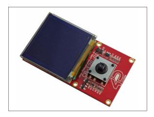
The **CB-128-G1** is a compact carrier board designed to provide a simple means of adding user input to the already capable uOLED-128-G1(SGC) (Serial Platform) and the uOLED-128-G1(GFX) (4DGL Platform) range of intelligent display modules. The tiny 5-position joystick, along with an on-board speaker, facilitates user input and output for these displays.
