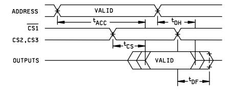
FIGURE 5. AC read timing diagram.
