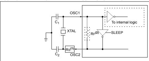
**Note 1:** A series resistor, Rs, may be required for AT strip cut crystals. **Note 2:** The feedback resistor, RF, is typically in the range of 2 to 10 M $\Omega$ .
