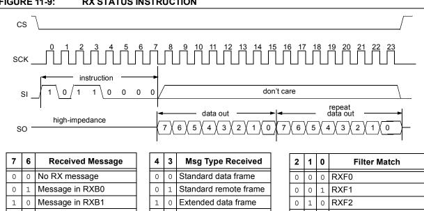
Messages in both buffers\* CANINTF.RXnIF bits are mapped to bits 7 and 6.
