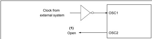
Note 1: A resistor to ground may be used to reduce system noise. This may increase system current.
