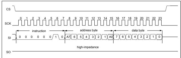
FIGURE 11-5: LOAD TX BUFFER
