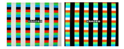
The same 2 patterns are also useful when sending video over UTP cable, such as Cat5, Cat5E or Cat6, both for the high-frequency loss and skew compensation. The right and left edges of the RGB bars should line up vertically. This pattern provides convenient means for making this adjustment.
