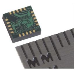
The HMC5843 utilizes Honeywell's Anisotropic Magnetoresistive (AMR) technology that provides advantages over other magnetic sensor technologies. The sensors feature precision in-axis sensitivity and linearity, solid-state construction with very low cross-axis sensitivity designed to measure both direction and magnitude of Earth's magnetic fields, from tens of micro-gauss to 6 gauss. Honeywell's Magnetic Sensors are among the most sensitive and reliable low-field sensors in the industry.
