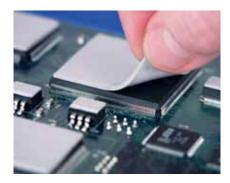
Gap Pad 2000S40 is recommended for lowstress applications that require a mid to high thermally conductive interface material. The highly conformable nature of the material allows the pad to fill in air voids and air gaps between PC boards and heat sinks or metal chassis with stepped topography, rough surfaces and high stack-up tolerances.
