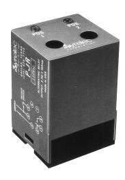
The electronic alternating relay is designed to replace mechanical style devices used in control applications requiring a duplexing or alternating action of the control circuits to operate pumps, compressors, etc. This is achieved by activating a control switch which is common to one side of the input control voltage. The output contact of the relay(s) change state when this switch is opened
