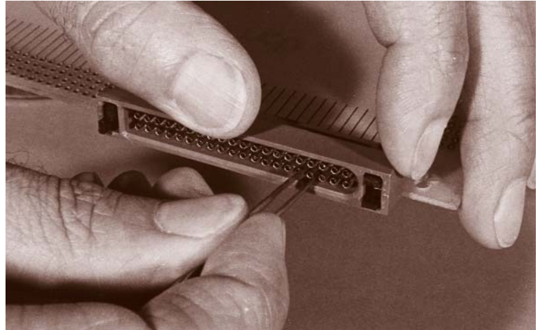
REMOVE DAMAGED CONTACT
