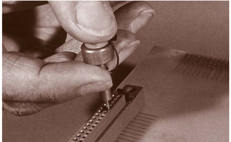
SEAT PLUNGER AND REMOVE CONTACT AND TOOL
