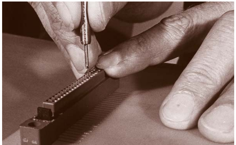
SEAT CONTACT WITH INSERTION TOOL
