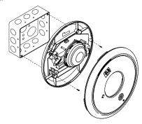
Genesis ceiling horn-strobes simply unlatch and twist to open. This gains access to mounting screws and the selectable candela switch. The shallow depth of Genesis devices leaves ample room behind the signal for extra wiring. Once installed with the cover in place, no mounting screws are visible.
