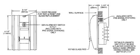
FLUSH INSTALALTION USING P-024900 STEEL BOX
