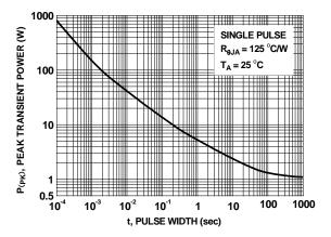
Figure 12. Single Pulse Maximum Power Dissipation
