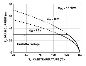
Figure 10. Maximum Continuous Drain Current vs Case Temperature
