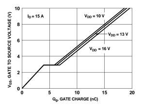
Figure 7. Gate Charge Characteristics
