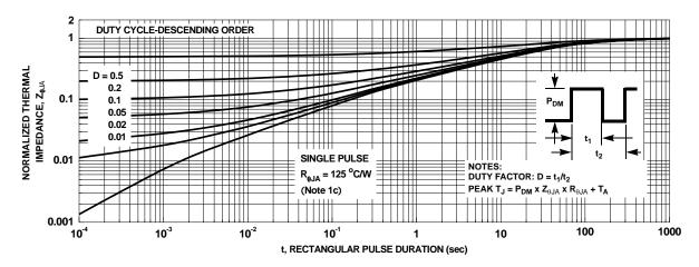
Figure 13. Junction-to-Ambient Transient Thermal Response Curve
