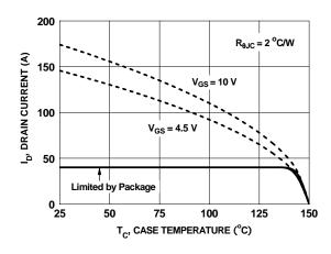
Figure 23.Maximun Continuous Drain Current vs Case Temperature
