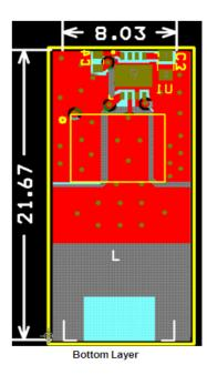
Figure 31. Recommended PCB Layout
