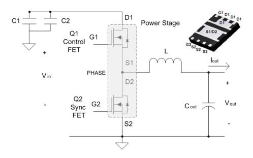
Figure 30. Shows the Power Stage in a buck converter topology
