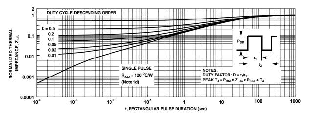
Figure 26. Junction-to-Ambient Transient Thermal Response Curve
