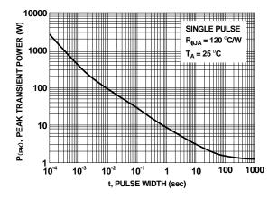
Figure 25. Single Pulse Maximum Power Dissipation
