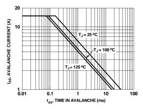
Figure 9. Unclamped Inductive Switching Capability
