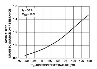
Figure 16. Normalized On-Resistance vs Junction Temperature
