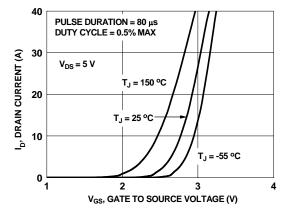
Figure 5. Transfer Characteristics
