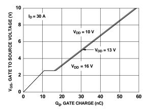
Figure 20. Gate Charge Characteristics
