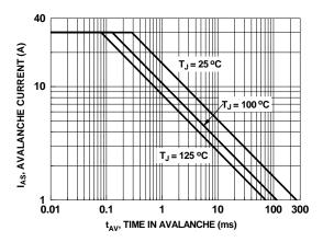
Figure 22. Unclamped Inductive Switching Capability
