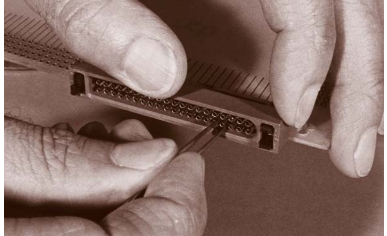
REMOVE DAMAGED CONTACT
