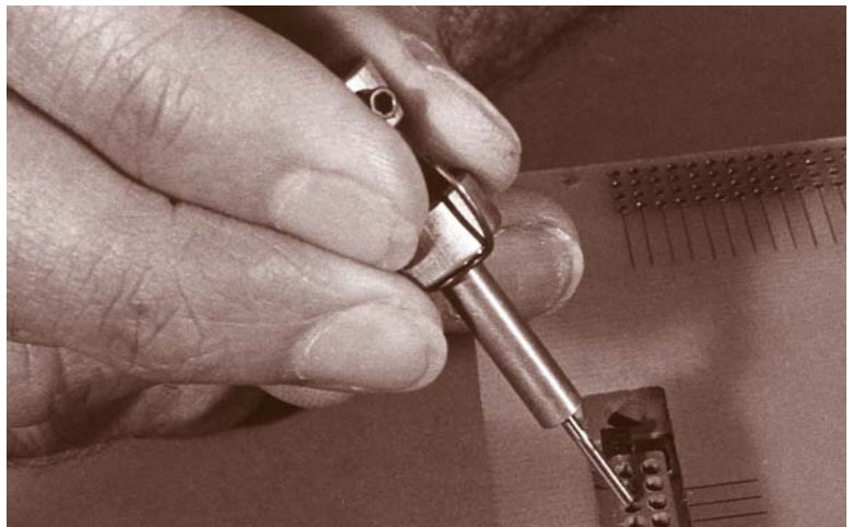
INSERT EXTRACTION TOOL WITH PLUNGER RETRACTED
