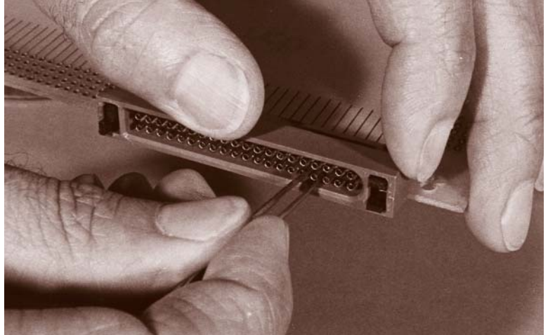
REMOVE DAMAGED CONTACT
