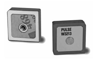
Pulse is please to announce the W3213 GPS patch antenna to compliment our growing range of tracking antenna products. This small  $0.5 \times .05$  inch  $(13 \times 13 \text{ mm})$  ceramic patch antenna is 0.16 inches (4 mm) high and has a pinthrough mount. Double sided tape is on the underside of the antenna for adhesion to the customer board.
