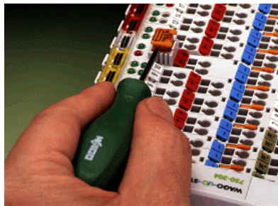
Fig. 2-15: Removing the fuse carrier
